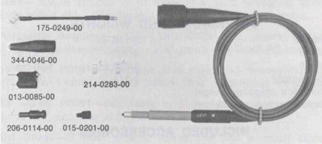
The P6057 is a miniature low-capacitance probe for use with 50  $\Omega$ , wide-band oscilloscopes. Bandwidth DC to 1.7 GHz. This probe can also be used with 50  $\Omega$  sampling systems, such as the 3S1 plug-in, or the S1 and S2 sampling heads, with a BNC male to GR adapter (017-0063-00).
