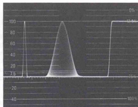
Fig. 1. Undistorted modulated  $\sin^2$  pulse.
