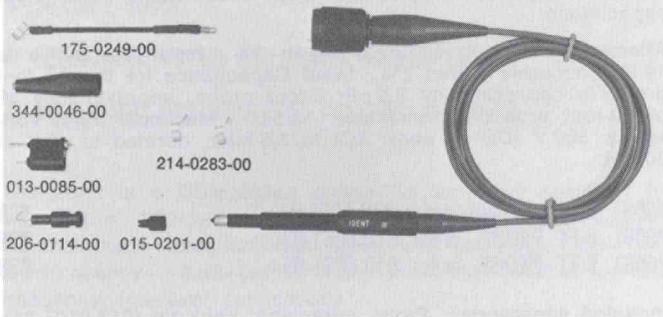
The P6056 is a miniature low-capacitance probe for use with 50  $\Omega$ , wide-band oscilloscopes. Bandwidth DC to 3.5 GHz. This probe can also be used with 50  $\Omega$  sampling systems, such as the 3S1 plug-in, or the S1 and S2 sampling heads, with a BNC male to GR adapter (017-0063-00).
