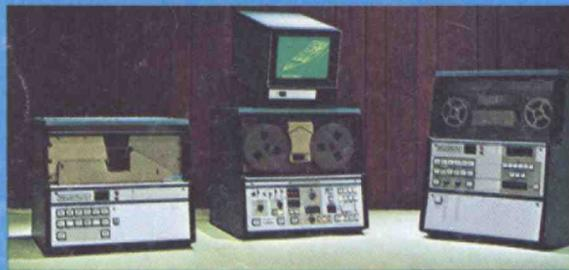
**AUTOMATIC TESTING SYSTEMS—**Automatic testing is an economical way to determine and maintain product quality. Tektronix, Inc. makes Functional, DC and Dynamic Testing Systems with features such as computer control, waveform digitizing, 20 MHz testing, instant graphing of results and hard copy option.
