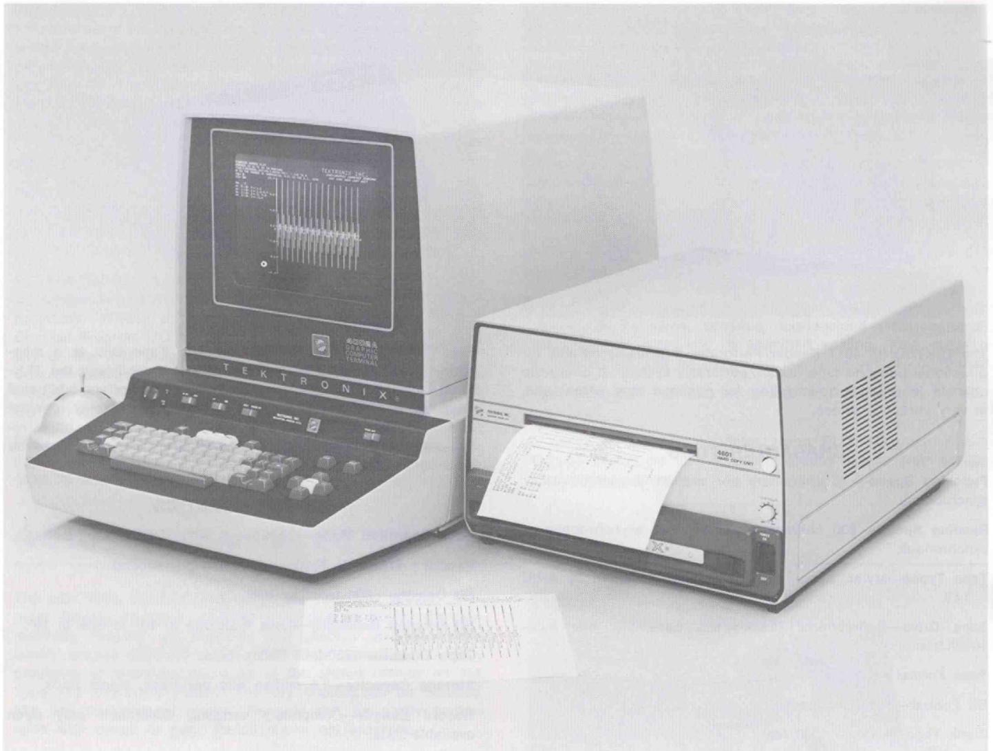
The 4002A is a self-contained, computer terminal which provides a high-resolution, flicker-free display of both complex graphics and high-density alphanumeric.
