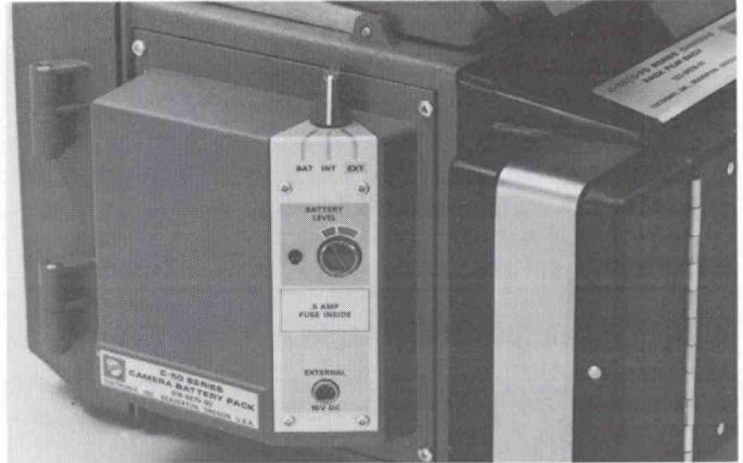
Optional battery pack installed on C-53-P Camera
