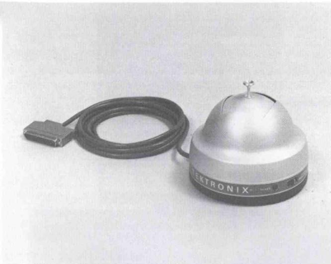
The 4951 Joystick inputs signals to the TEKTRONIX 4902 Interactive Graphic Unit. These signals provide the X and Y information for positioning the cursor generated by the inter-
