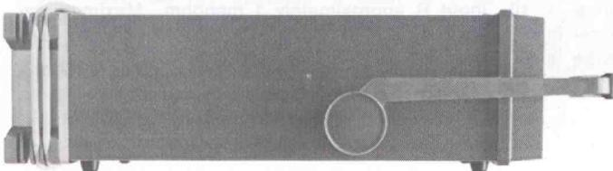
**Amplitude and Time Calibrator**—0.6 V adjustable within 0.5%. Repetition rate is adjustable to 1 kHz within 0.25% ( $+20^{\circ}\text{C}$  to  $+30^{\circ}\text{C}$ ). Output resistance is 575 ohms.
