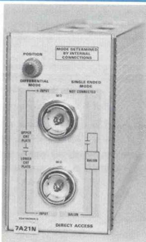
The 7A21N plug-in is designed specifically for the AC coupling of high frequency or fast risetime signals directly into the wide bandwidth CRT of the 7904 Oscilloscope. Two front panel input connectors allow either single-ended or differential operation (internally selected). Vertical trace positioning is accomplished by a front panel control.
