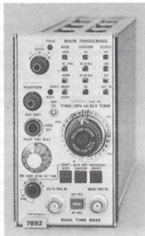
The exceptionally fast sweep (500 picosecond/cm) of the 7B92 ideally matches the ultra-high bandwidth of the 7904 mainframe. The 7B92 features four display modes: normal, intensified delaying sweep (controllable contrast), delayed sweep and alternate.
