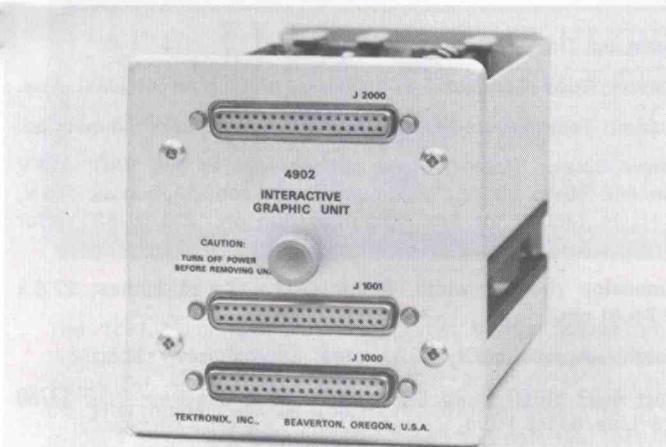
The 4902 interfaces the 4002A Computer Display Terminal with graphic input devices.
