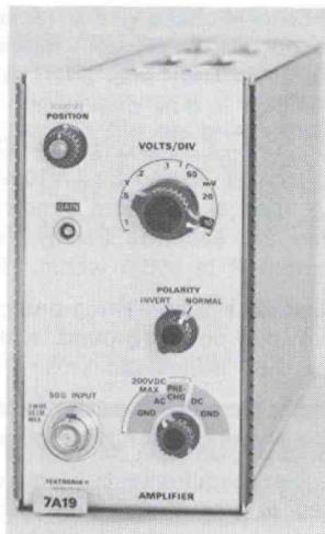
The 7A19 is a high performance, wide bandwidth, single-trace plug-in amplifier designed primarily for use with the 7900-Family mainframes, but is compatible with all 7000-Series mainframes. The polarity of the display is selectable, either normal or inverted. As an option the 7A19 is available with a variable (front-panel) delay line to permit matching the transit time of two preamps and probes to better than 50 ps. The range of this variable delay is  $\pm 500$  ps.
