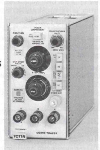
The 7CT1N Curve Tracer is a plug-in unit used in TEKTRONIX 7000-Series Oscilloscope Systems for displaying characteristic curves of small-signal semiconductor devices to power levels up to 0.5 watts.
